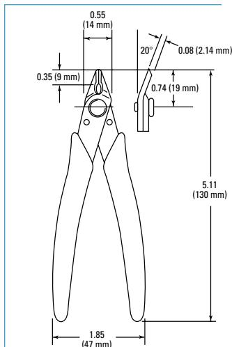
170-II Series shears offer numerous ergonomic enhancements in an "economically priced" tool. Their effort-reducing Micro-Shear® cutting action requires only about half the effort to cut a wire as that required by conventional compression-type cutters. The 170-II Series feature advanced ergonomic shape, Xuro-Rubber™ grips, a glare eliminating black finish, light weight and our patented, lifetime warranted, *Light Touch*™
