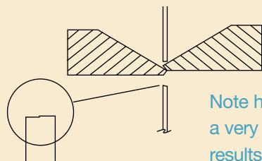
This is a cross section view of a XURON Micro-Shear® flush cutter from the tip end.
