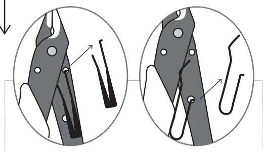
The spring style can vary between models. All styles have a tiny foot that hooks into one of the holes in the tool's handle.
