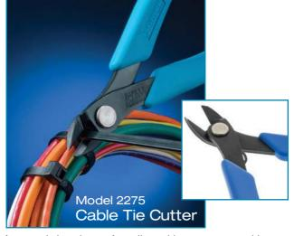
An extended cutting surface allows this cutter to cut cable ties as wide as  $\frac{1}{4}$  inch (7 mm). Micro-Shear® Flush Cutting blade bypass action leaves a flat end on the cut cable tie with no spike or pinch.
